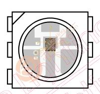
Model: HD107S 5050-RGB 40MHz Clock Drive Frequency
